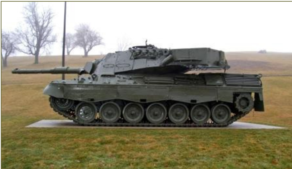
Similar Leopard C2s (Leopard C1A3 upgraded with the addition of a Leopard C1A5's turret) are currently being used in Afghanistan in counter-insurgency operations. Photo taken at the Royal Military College by the author.
