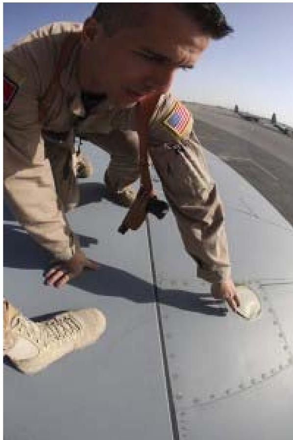
**That little membrane tears off and reveals a handle for the life raft, which pops out of the wing just behind Gabe's left arm.**
