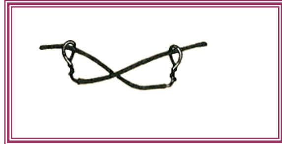
Figure E-7: Pull-Loop Switch (Source: TM 31-210)
