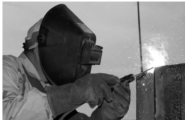
SGT Clay O'Dell, 3-112th Armor Battalion, 56th Brigade Combat Team, 36th Infantry Division, welds a 3/8-inch steel armor plate on a HMMWV in southern Iraq.
