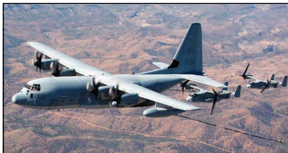
A VMGR-252 KC-130J performs aerial re-fueling of MV-22s over the Southwest desert
