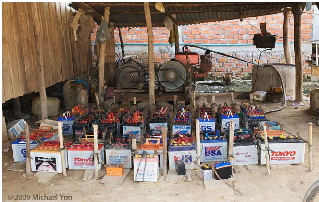
Cambodia: Light in many homes is provided only by battery. A small business that uses a generator charges the village batteries. If a traveler needs a satphone or cell phone charged, they must only find one of these places and a local will charge your batteries while you have tea. In some places, including Iraq, people charge cell phones on motorcycles.
