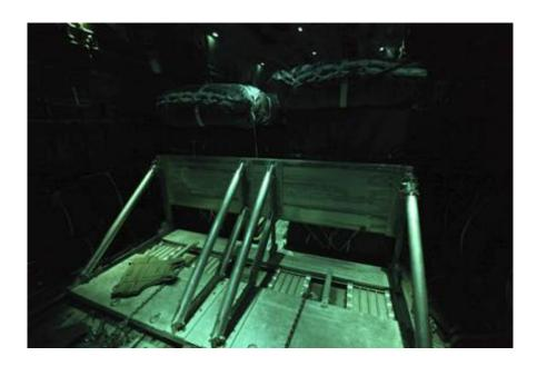
**9188a** - This is the BSA, or Buffer Stop Assembly. The BSA is designed to keep the cargo from lurching forward during flight.
