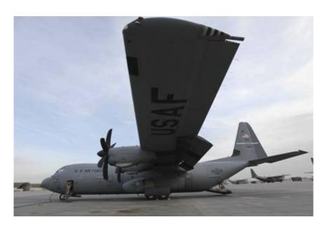
**8872** - The latest and greatest for general use is the C-130J. You can spot a "J" from the older variants by looking at the propellers. Each propeller has six high-tech blades, allowing the
