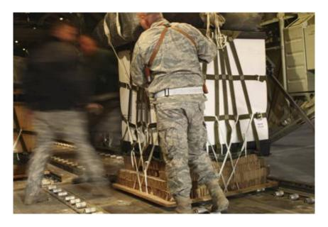
**9081**- In addition to the loadmasters heavy responsibilities, the riggers who "build" these pallets and attach the parachutes must be on their job. They call this a CDS, or container delivery system, and they said it's using LCADS "low cost air delivery system" parachutes that are
