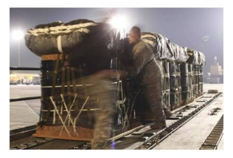
**9083a** - Atop are the LCADS parachutes, and these are fuel drums. Usually, our people try to avoid parachuting ammunition in Afghanistan. Though normally right on target, cargo has a real chance of floating into enemy hands. Also, ammo is more easily damaged than MREs and fuel.
